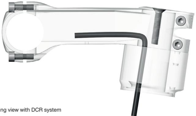
Fig. 4.3.2: cable routing view with DCR system
